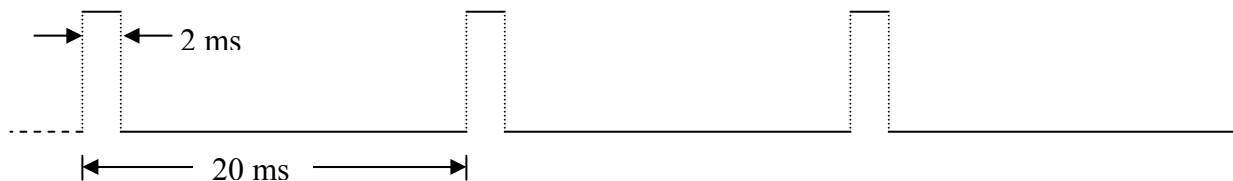
Figure 1: Pulse waveform with 10% duty cycle
