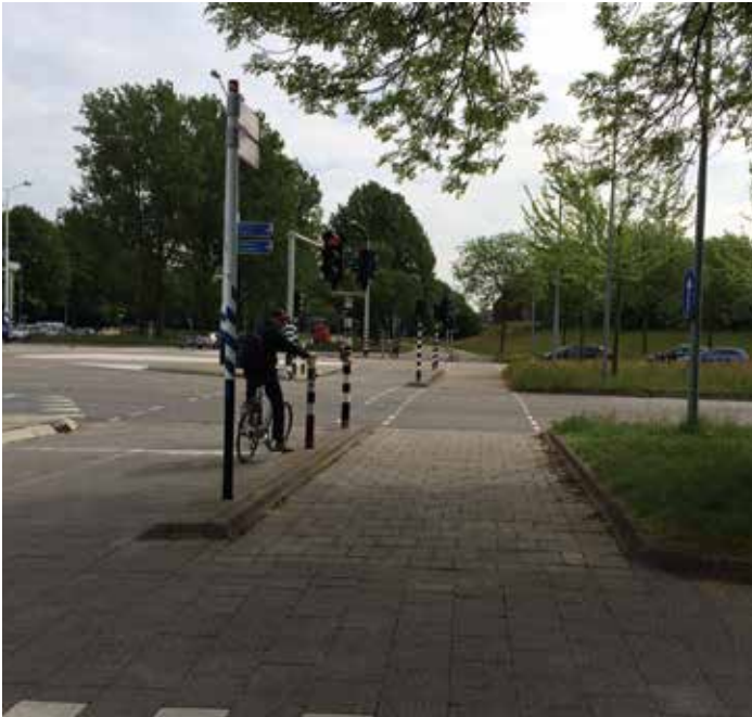
Separated Bike Lanes and Integrated Signalization
