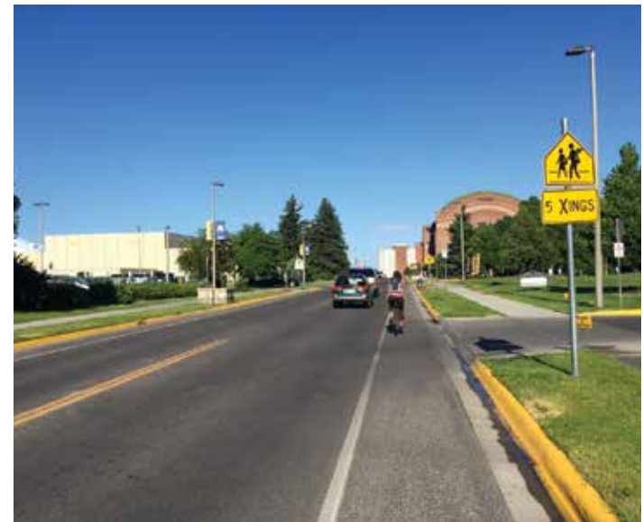
This bike lane on Grant Street is unmarked other than the edge line
