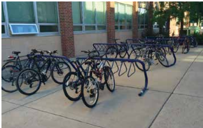
The CORA, or coat hanger, rack is free standing and supports a bike in two places if used correctly
