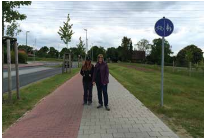
Separated bike path in Munster, Germany. Pedestrians use the right side of the path and bicycles use the left (red pavement)
