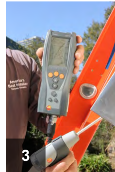
Verify that carbon monoxide levels are within specifications
