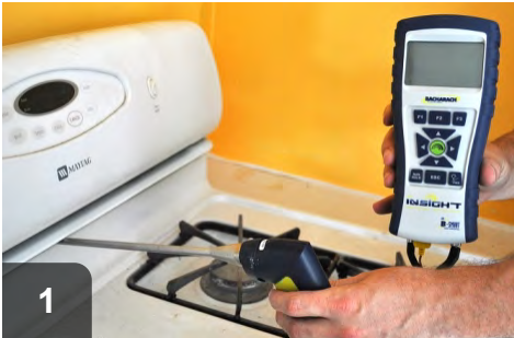
1 Test for CO in entire home, particularly around combustion appliances
