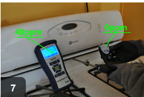
7 After mitigation, verify that CO has returned to safe levels
