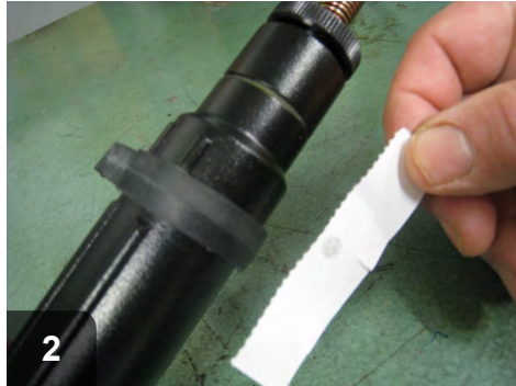
Remove paper and verify draw was successful by checking for soot
