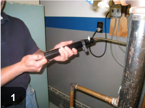
Place filter paper in testing pump and draw air through paper
