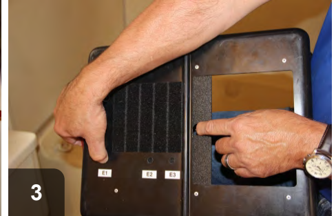
3 Adjust gate on the flow meter as needed.
