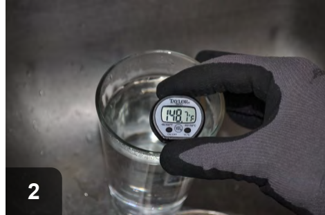
2 Hot water temperatures should not exceed 120 degrees Fahrenheit
