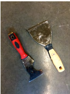
Scrape loose material from insides of cabinet
