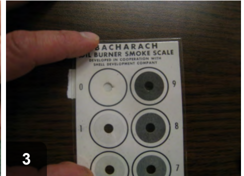
Compare level of soot deposit against smoke chart. A rating of 0 is ideal
