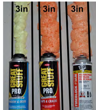
Spray foam can be used to span gaps up to 3 inches
