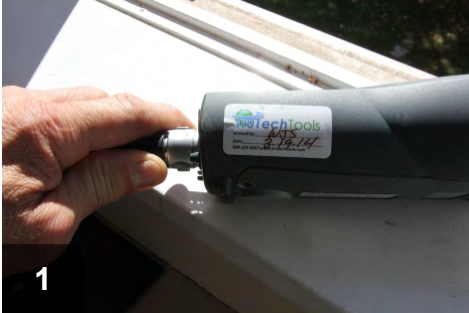
Verify that calibration date is current on combustion analyzer
