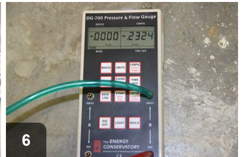
Measure resulting pressure drop of the dry evaporator coil.
