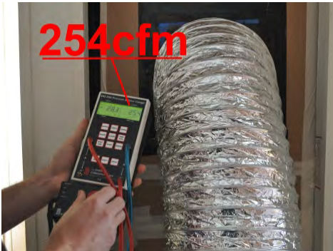
Perform duct blaster testing before beginning work. Record results
