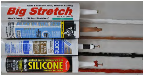
Caulking can be used to span gaps up to 1/4 inch
