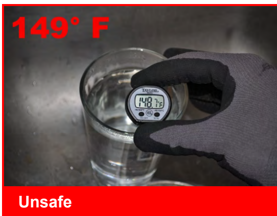
Hot water temperature over 120°F
