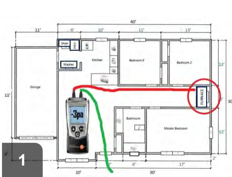
1 Run depressurization testing on house to ensure new ventilation isn't causing unsafe conditions
