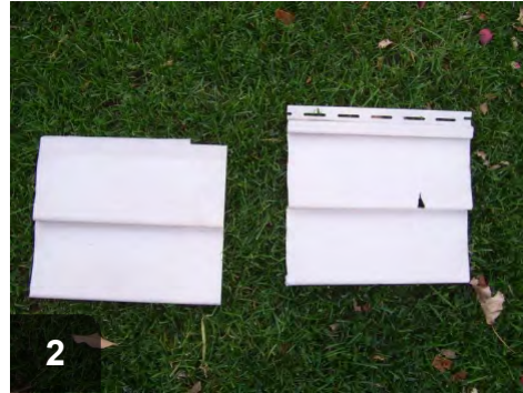
Use siding that matches the existing material's contour, texture, and color
