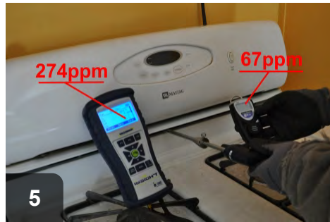
5 When cause of elevated CO levels has been located, take steps to correct
