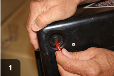
1 Attach hose to the fan meter.
