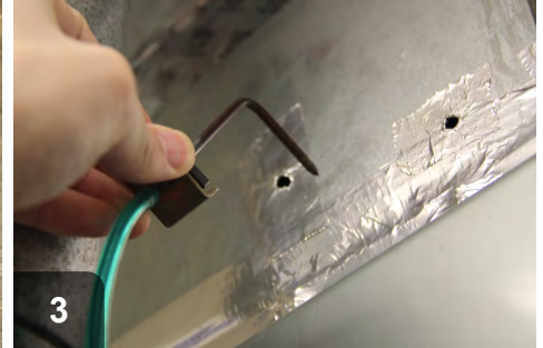
Static pressure probe should be inserted with the tip pointing into the air stream.
