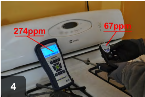
4 When cause of elevated CO levels has been located, take steps to correct
