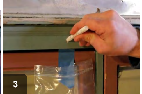
3 Break capsules and shake to mix reagents. Swab sample site for 30 seconds
