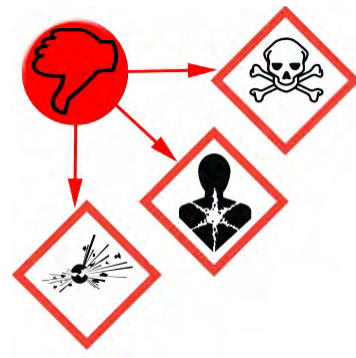
Do NOT use hazardous materials in confined spaces -- particularly those carrying these GHS warnings
