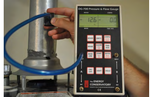
Complete draft test using a manometer
