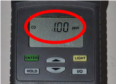
CO levels cannot exceed 100ppm, or 200ppm air-free CO
