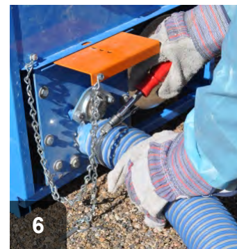
If testing shows machine is operating properly, attach hose and tighten fitting to minimize slippage
