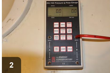
2 Attach hose to the manometer set to PR/PR.
