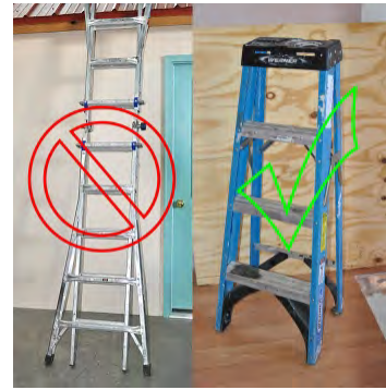
Use fiberglass ladders in place of metal
