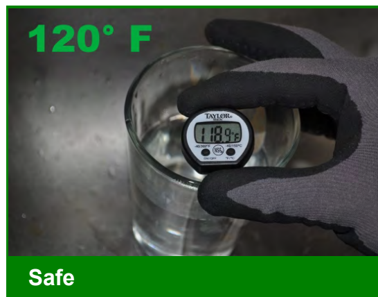
Hot water temperature under 120°F
