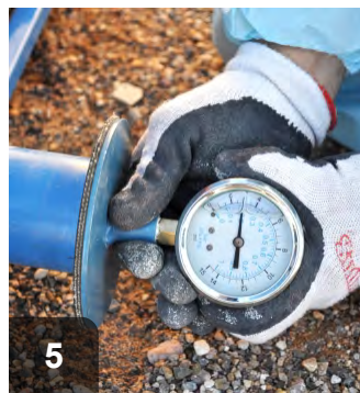
Using pressure gauge at feed outlet, verify that machine is working within manufacturer's specifications
