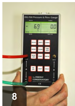
8 Manometer reading should be within allowable limit (See 2.0299.1a-i)
