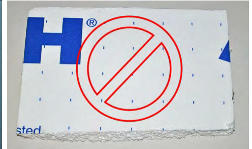
Do not use EPS (expanded polystyrene) foam board in floor cavities due to flame spread rate
