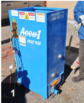
Set-up blowing machine on dry, level surface near electrical source and insulation site
