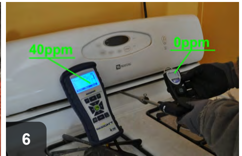
6 After mitigation, verify that CO has returned to safe levels
