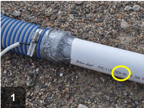
Select rigid fill tubes that are low conductivity -- Schedule 40 PVC fill tube
