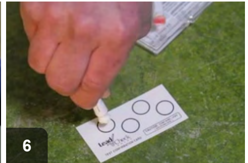
6 If negative, verify validity of test with provided calibration card
