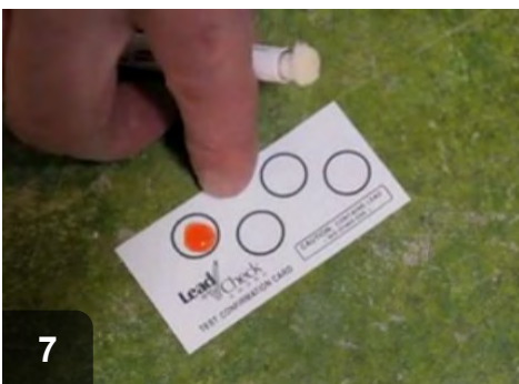
7 Lead in calibration card should test positive and turn red
