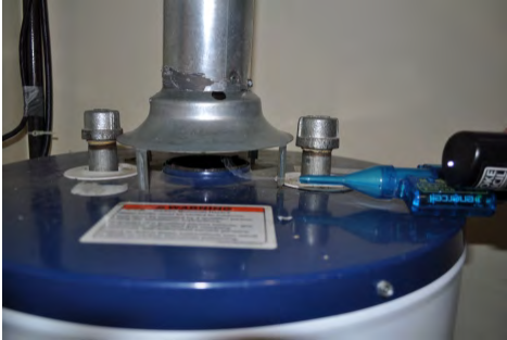
Complete spillage test using chemical smoke pencil
