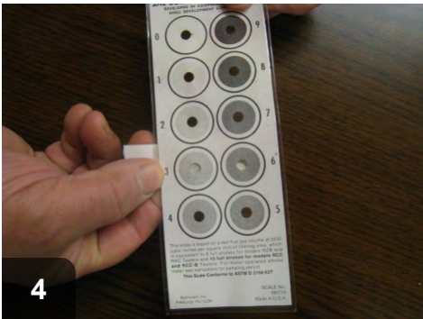
Appliances with ratings of 3 or higher should be cleaned and tuned
