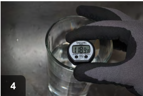
4 After adjustment and insulation, retest to verify temp is under 120 degrees
