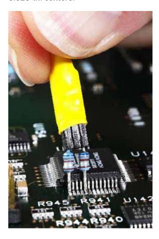
The coaxial resistor is able to make contact with an individual package lead without bridging over to adjacent pins. The illustration shows a closer view of the electrical connection.
