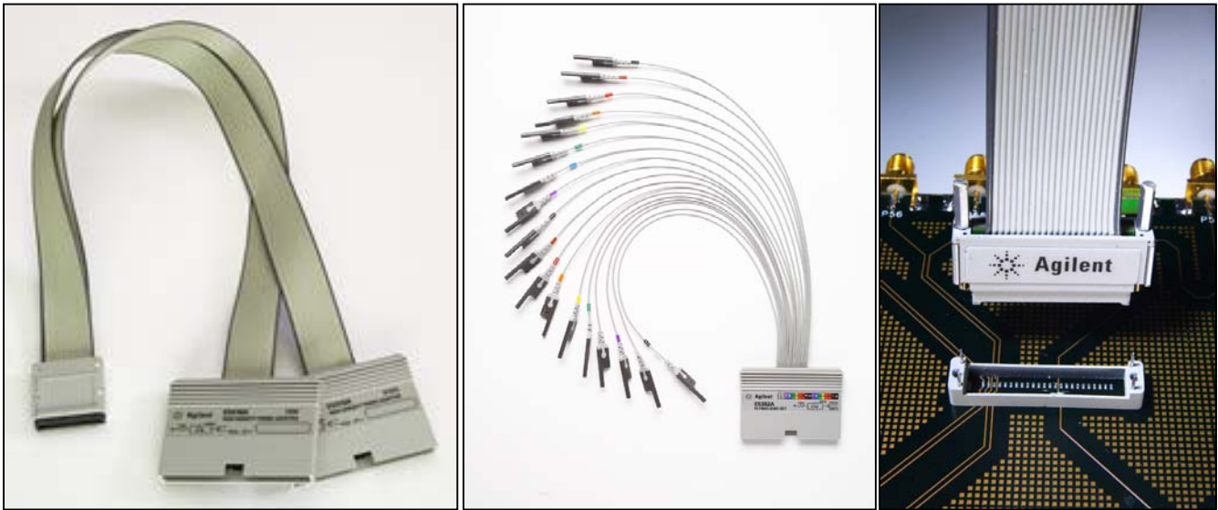
Figure 27. Modern Probing Solutions (Connector-Based, Flying Lead, and Connector-Less)
